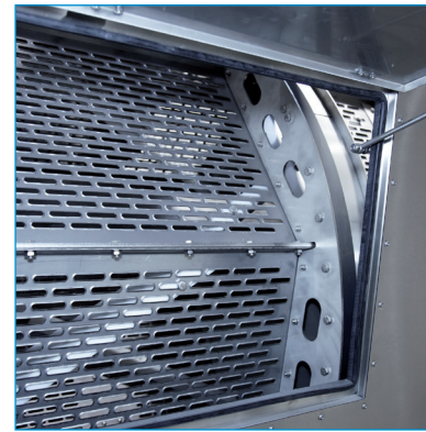
Washing drum | stainless steel Waschtrommel | rostfreier Stahl
