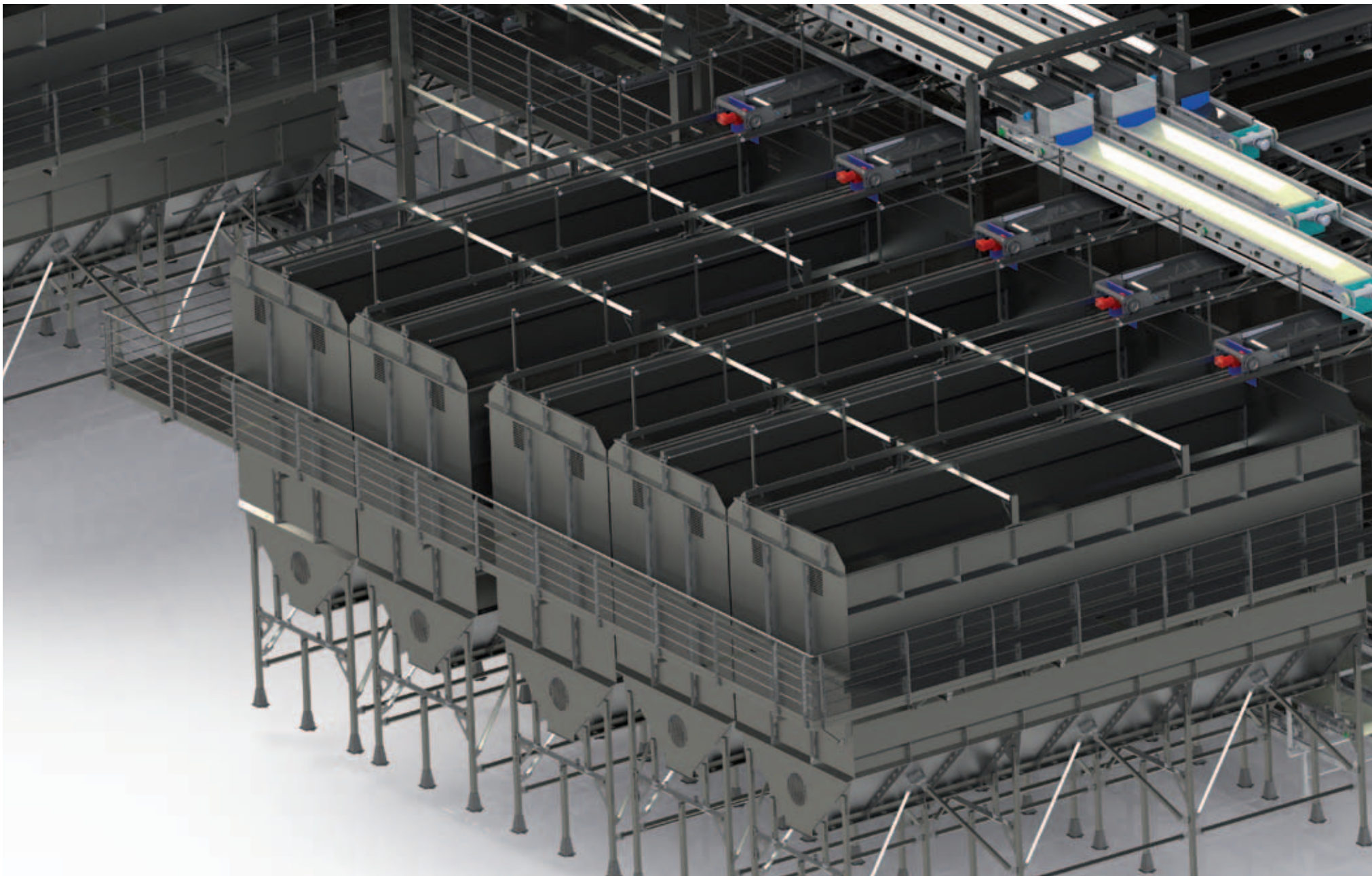
USA | Plant design | Detailed view of the storage system for french fries USA | Anlagenplanung | Detailsansicht des Lagersystems für Pommes Frites
